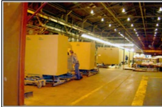
In addition, CAVS-E engineering designed and supervised the construction of a *cab trim and assembly moving* assembly line that proved to be an effective and innovative approach to KBR Cab production. The final assembly line (Figure 10), was located inside Bay 1 and was fully equipped with electrical, compressed air, and high-intensity lighting for cab interior trim and assembly.
