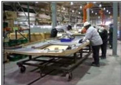
Bay 1 was completely reconfigured from the old KBR armored cab layout and was fully equipped during the early MaxxPro® ramp-up. Major installations included light-rail overhead crane systems, a single-line in-floor conveyor system, high-intensity lighting, multiple-voltage electrical outlets, and high-speed internet connections.
